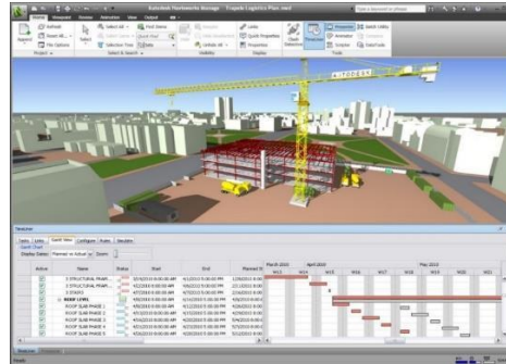
Figure 4. Integration of BIM models and project management models and 4D model production
